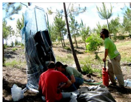
oio- Sprinkler Rainfall Simulator developed by Cerdà
