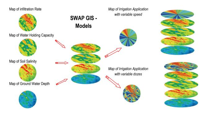
Framework to develop maps of irrigation applications of variable rate irrigation technologies
