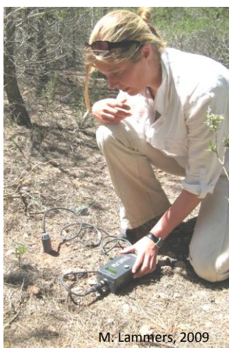
Measuring soil moisture content
