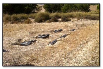
Storage tanks (left) and runoff collectors on adjacent open plots (upstream to the right)
