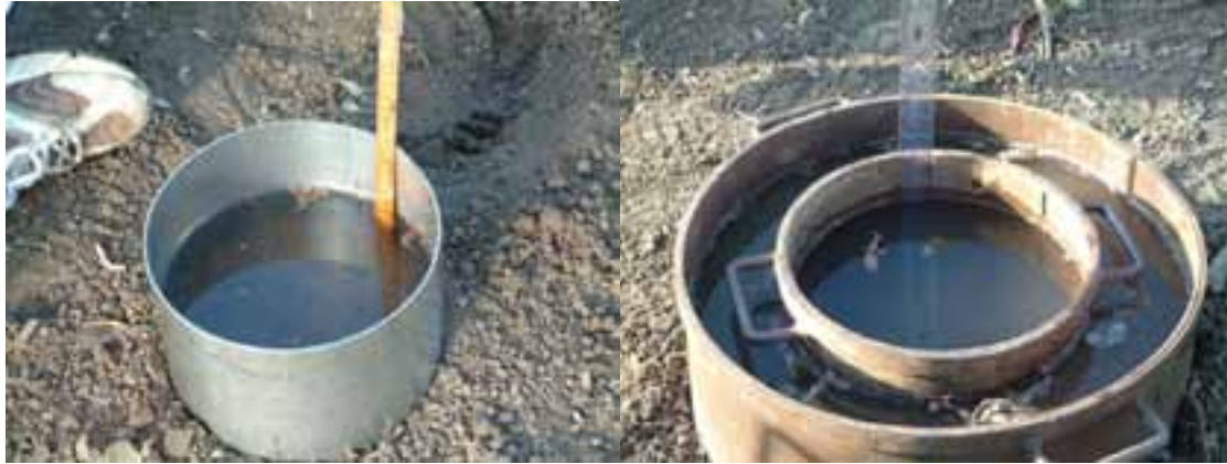
Figure 5.4. Left: single ring and right: double ring infiltration test. Here the water levels are not controlled by a Mariotte bottle an need to be carefully maintained. This is only possible for soils with a low infiltration rate (photo: http://en.wikipedia.org/wiki/Infiltrometer )
