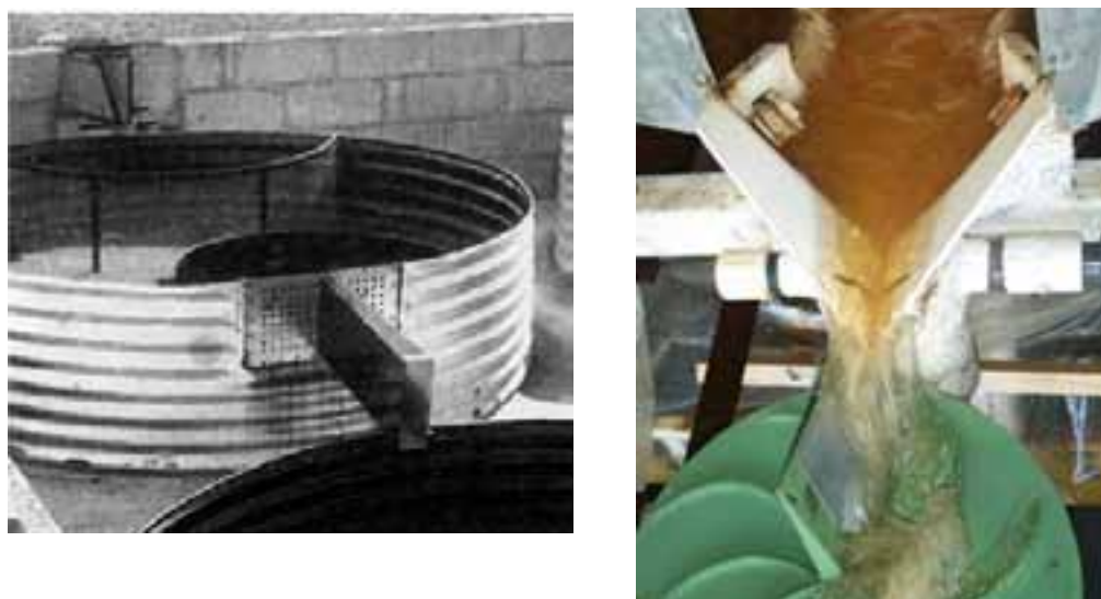
Figure 7.7. Sediment sampling: multislot divisor (left, Hudson, 1993)) and Coshocton wheel (right, USDA North Appalachian Exp. Watershed website)).
