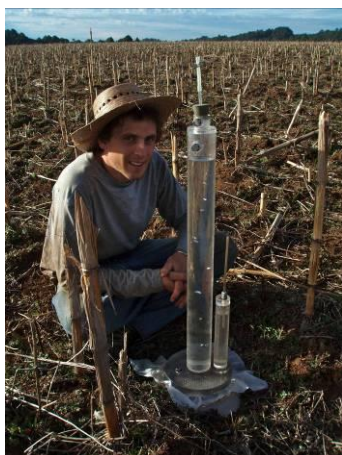
a/ Youen Grusson with the disk infiltrometer on Andosol corn field let just harvested (C. Prat 27.04.10) b/ C. Prat and Y. Grusson doing measures with disk infiltrometer on Andosol corn field let in fallow (P. Bustos 2010)
