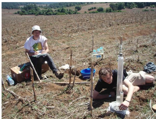
a/ Youen Grusson with the disk infiltrometer on Andosol corn field let just harvested (C. Prat 27.04.10) b/ C. Prat and Y. Grusson doing measures with disk infiltrometer on Andosol corn field let in fallow (P. Bustos 2010)
