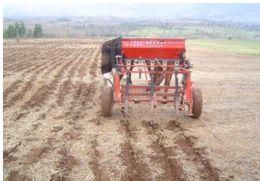
Zero tillage machine drawn by oxen. Seeding of lentils in the rainfed area of Ninhue County . Photo by Carlos Ruiz
