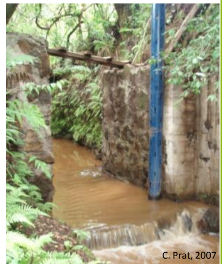
Measuring sediment and discharge in channels
