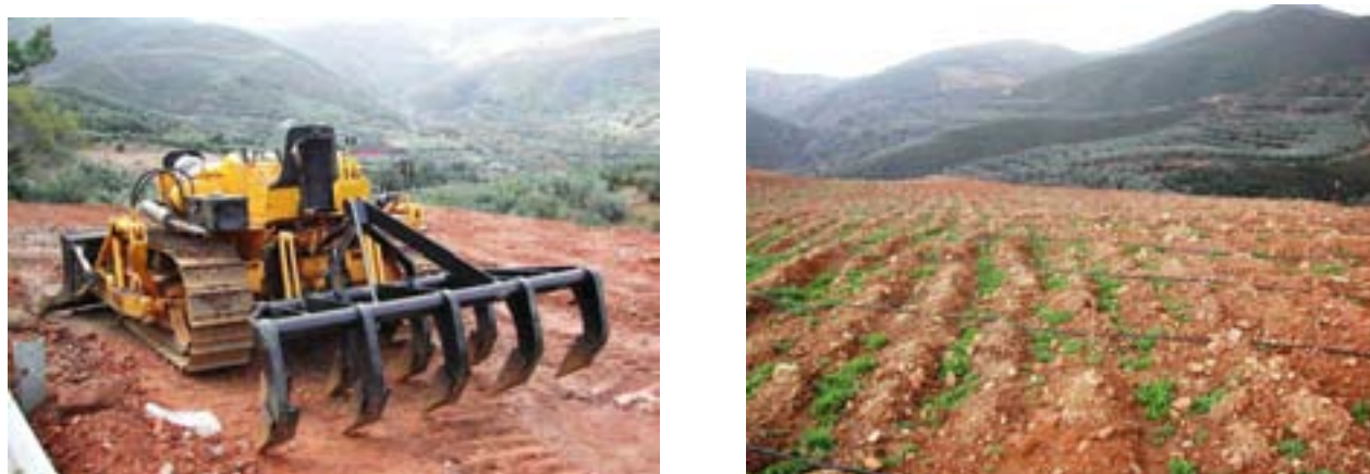
Fig. 57. Tillage implement used for cultivation of hilly areas (left) preparing the soil for planting (right)
