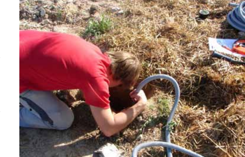
Installing soil moisture sensor
