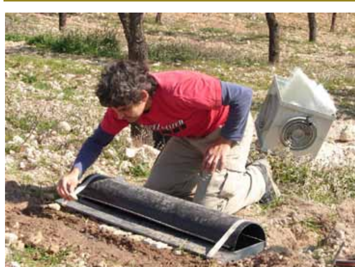
Installing Gertlach plots
