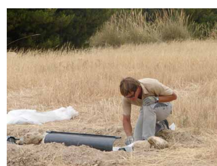
Installing runoff and erosion plots under cereal
