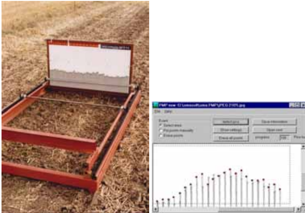
Figure 6.7. In situ semi-automated pinmeter and an application for analysing pinmeter measurements (REF)
