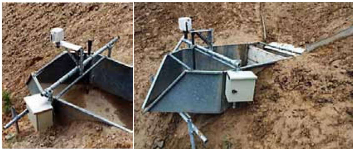
Figure 8.4. Small flume with ultrasonic water level sensor and turbidity sensor built into the hillside slope at the bottom end of the gully (photo Erochina project ALTERRA).
