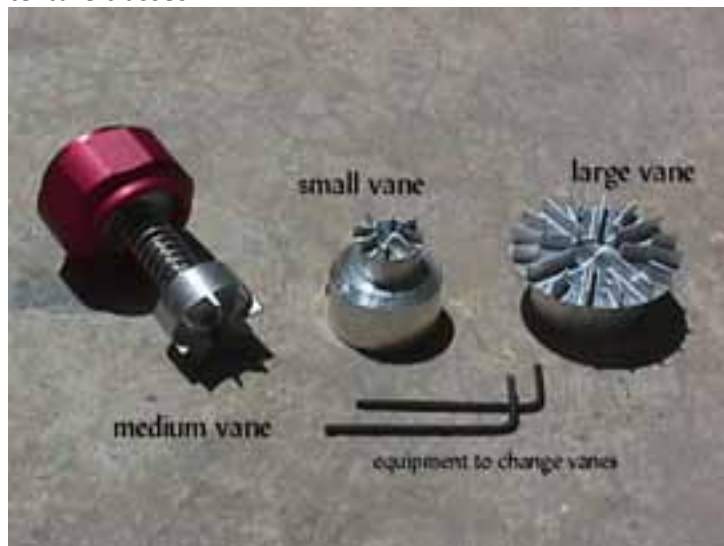
Figure 5.7. Pocket shear vane with various disks for different types of soils: sand requires larger disks, clay requires the smaller disk.
