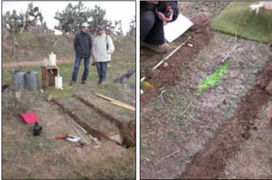
Figure 6.9. Manning's n measurements in Morocco, left general setup, right dye tracer injected in flow (photo V. Jetten).
