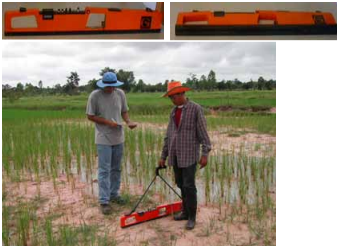
Figure 11.2. Top: EM38 in vertical (V) and horizontal (H) modes, bottom: use in the field
