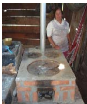
Figure 4.2.5: Wood saver rural oven (« patsari » model) (Photo: E. Rios, SEMARNAT)
