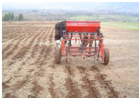
Figure 4.6.2: Zero tillage machine tractioned by oxen. Seeding of lentils in the rainfed area of Ninhue County (Photo by Carlos Ruiz)
