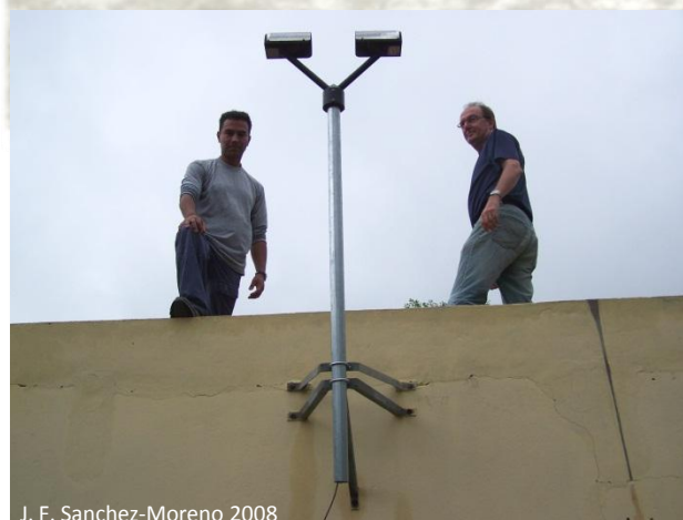
Optical disdrometer for measurement of raindrops
