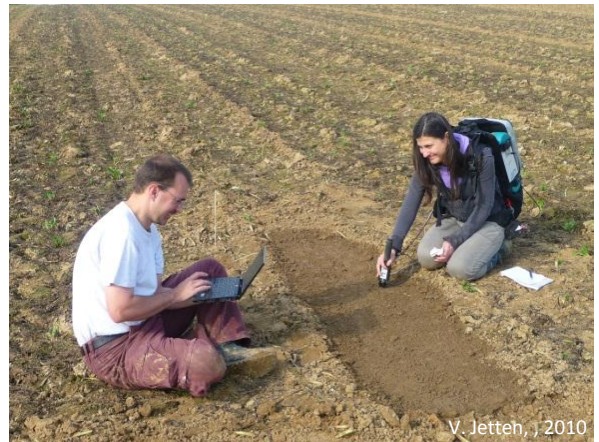
ASD Spectrometer measurements, South Limburg
