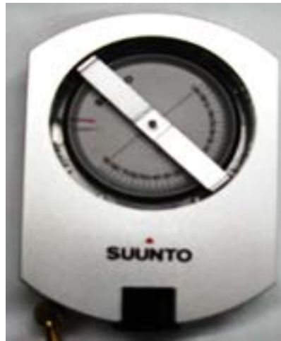
Fig. 13. Clysometer used for measuring slope gradient of a land surface
