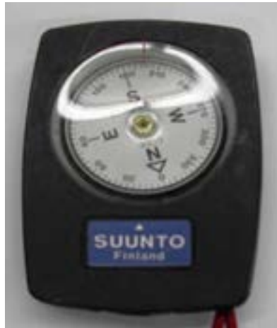
Fig. 12. Compass for assessing the relative earth's surface with respect to the magnetic north
