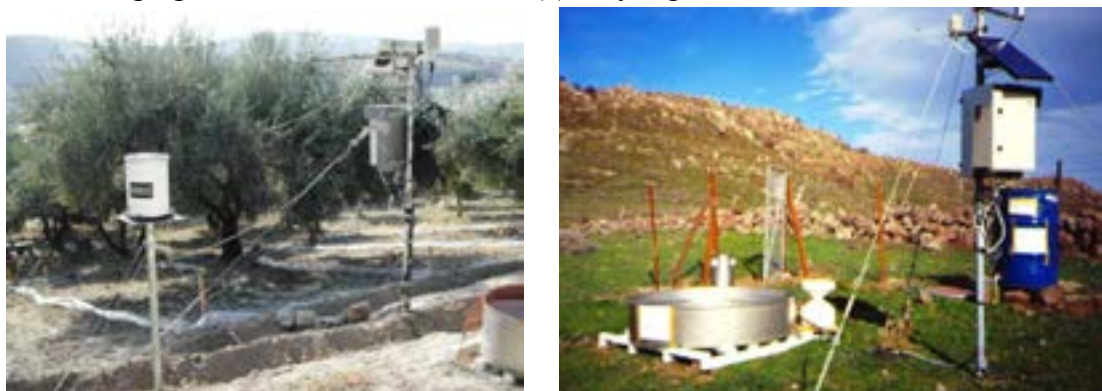
Fig.2. Automatic meteorological stations for collecting meteorological data for calculating evapotranspiration
