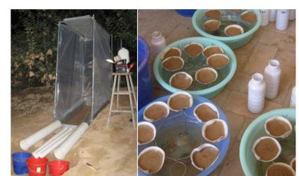
Building erosion plots on the slope of orchard in Miaowan village (2 gradients ,13 and 29), 5 meters long, three treatments (natural slope without coverage, contour tillage and contour with mulching, two times) . Some soil erosion tests with simulating rainfall finished.
