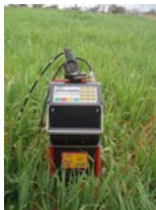
Photo 2. Soil water content measurement with neutron probe
