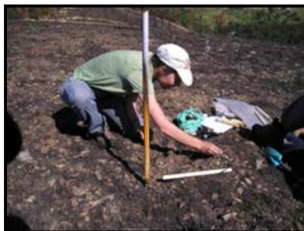
Fig. 4: experimental design of the soil water repellency grid (left); and measurement of hydrophobicity at five points, along a mini-transect (marked by the white tube), in the burned grid, at Vale Torto, in march 2009 (photo).
