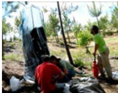
Figure 7 - Sprinkler Rainfall Simulator developed by Cerdà
